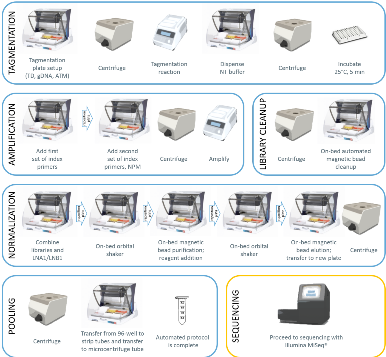
Figure 2: Schematic representation of the five PIPETMAX® scripts for automation of the Nextera® XT System DNA Library Kit workflow. Each blue rounded rectangle represents one PIPETMAX® script, each of which corresponds to a portion of the Nextera® XT System workflow. Some scripts include repositioning the plate or off-bed steps accomplished through user intervention, such as centrifugation of a microplate between liquid handling steps.
