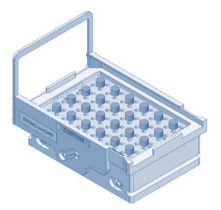
**Figure 2:** The custom magnetic bead separator (part number SPL2294) contains 24 magnets which can be raised or lowered to be in close contact with a 96 well plate. Each magnet is positioned between four wells, pulling the magnetic beads to the corner of each well.
