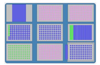
**Figure 4:** User interface for bed layout on PIPETMAX<sup>®</sup>. Labware and reagents from left to right, back to front: Tip Waste Chute, DSF200ST Tip Rack, DSF200ST Tip Rack, RSB Resuspension buffer in 0.2mL 8-Tube Strips, empty MIDI plate for final eluted libraries, liquid reservoir containing AMPure<sup>®</sup> XP beads and 80% Ethanol, starting material (amplified Libraries, DSF200ST Tip Rack, and another empty MIDI plate on the magnetic bead separator for the clean-up procedure.
