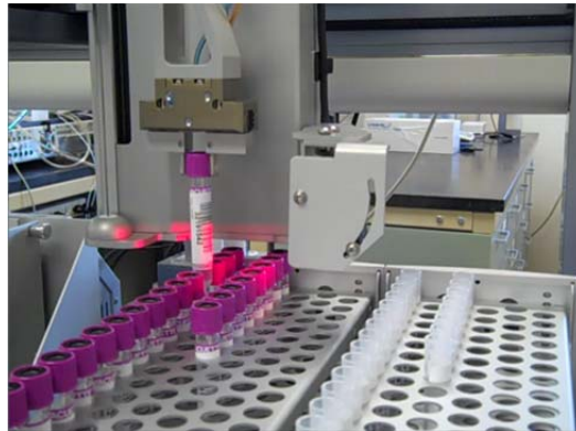
Figure 1. Gilson GX-281 equipped with a barcode scanning system
