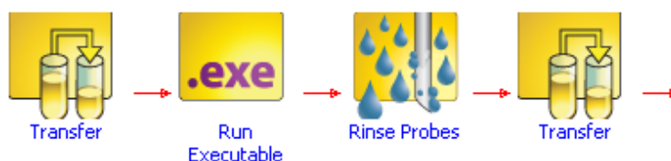
Figure 6. TRILUTION LH Method to Trigger the Agilent 8453 Spectrophotometer
