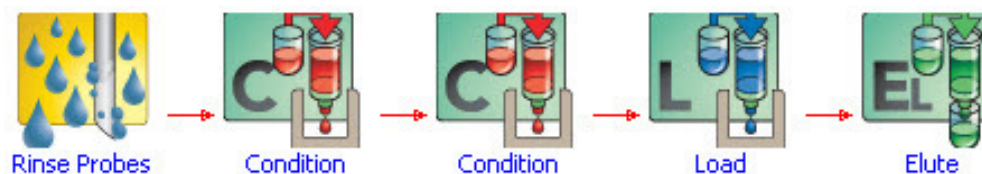
Figure 2. TRILUTION LH Basic SPE Tasks for Solid Phase Extraction of Lamotrigine and Metabolite from Water
