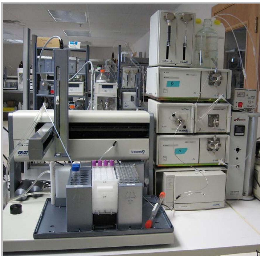
Figure 3. Gilson GX-271 Liquid Handler with 402 Dual with Tee Syringe Pump, 306 Mobile Phase Pumps, and a 152 UV-VIS Detector.
