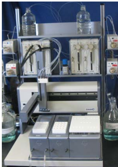
Figure 1. Gilson Large-Volume Clean Water Solid Phase Extraction System (GX-274 ASPEC System Base With Special 1931-Series Accessories & Operated Using TRILUTION® LH Liquid Handling Software).
