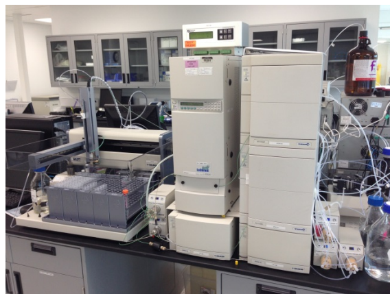
Figure 1. Fully Integrated and Flexible Oligonucleotide Purification System. A Gilson GX-271 Prep Liquid Handler was equipped with two GX Direct Injection valves and integrated with 322 Binary Mobile Phase Pumps, several ValveMates, 152 UV/Vis Variable Wavelength Detectors [0.2 mm Flow Cell (Prep and Desalting); 5 mm Flow Cell (Analytical)], Hitachi Elite LaChrom L-2350 Column Oven, and Pharmacia Biotech Conductivity Meter. The complete system was controlled with Gilson TRILUTION® LC Software.
