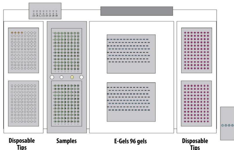
**Figure 1: 735 Sampler Software Tray File for the Quad-Z 215 with Disposable Tips and the Custom Rack Code 778 for the E-Gel 96 gels**
