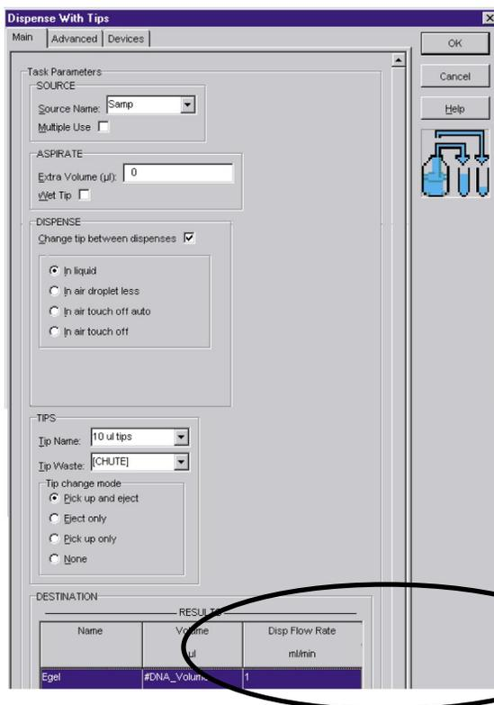
**Figure 2: 735 Sampler Software Task Used to Dispense the Sample into the E-Gel® 96 gels**
