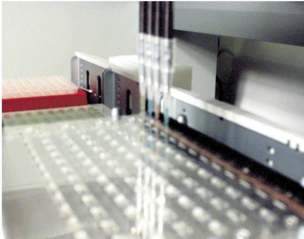
**Photo 3: Quad-Z 215 with Disposable Tips Accessing the E-Gel 96 gels**
