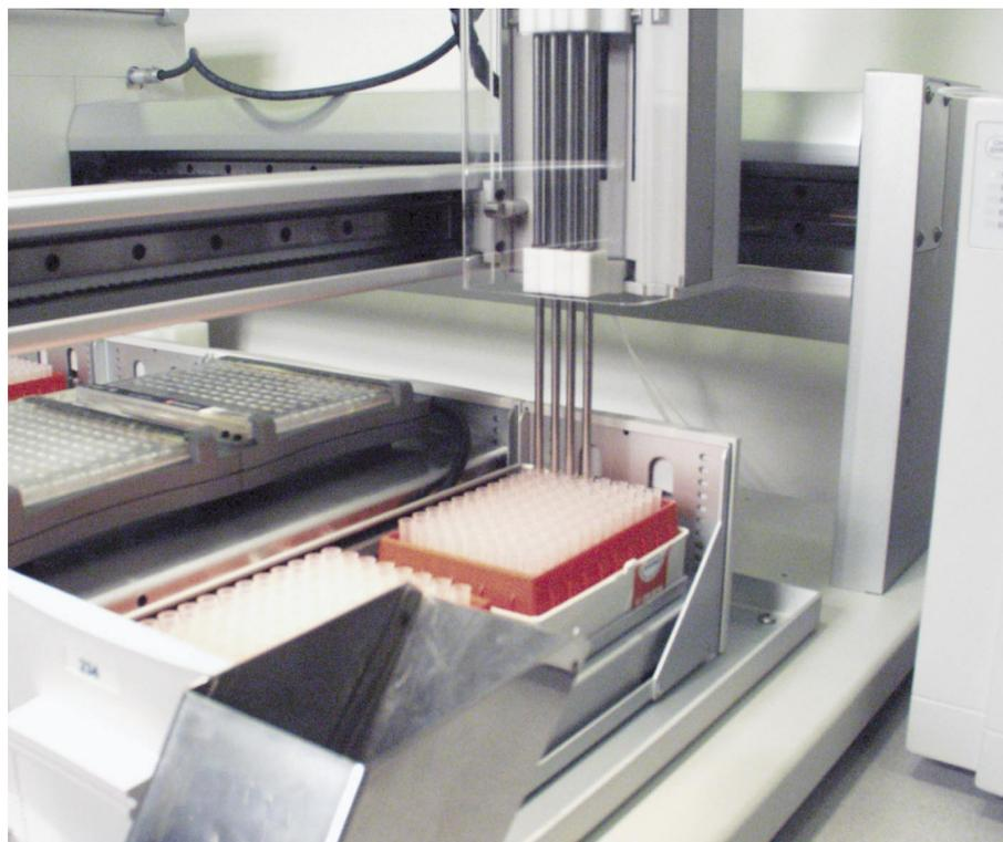
**Photo 2: Quad-Z 215 Picking Up 10-µL Disposable Tips Prior to Sample Aspiration**
