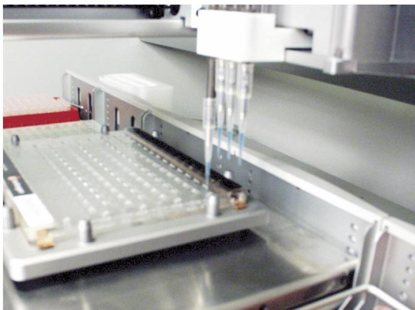
**Photo 5: Quad-Z 215 with Disposable Tips Demonstrating Independent Control to Access the Last Marker Lane**
