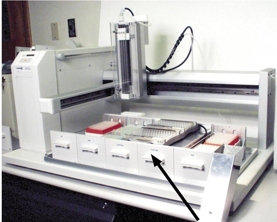
**Photo 1: Quad-Z 215 with Disposable Tips Fitted with Custom Rack Code 778 to Accommodate the E-Gel 96 Gels**
