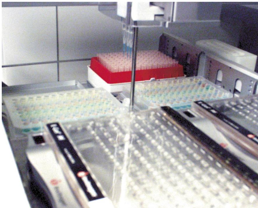
**Photo 4: Quad-Z 215 with Disposable Tips Demonstrating Independent Tip Movement**
