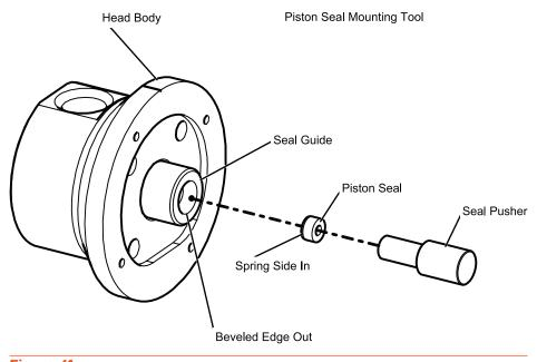
**Figure 41**Piston Seal Installation
