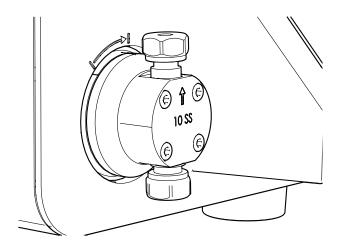
Figure 36 Pump Head Installation
