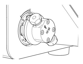
Step 3 Twist clockwise to install.
