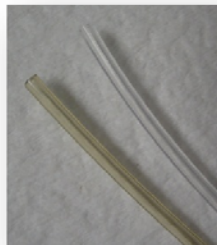
Figure 4: Transfer Tubing Radel R (left); - HPFA+ (right)
