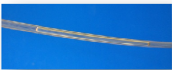
Figure 5: Radel R Tubing Showing Intact Air Gap
