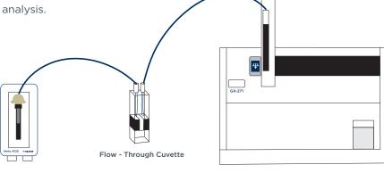
Figure 1 Sipper configuration
