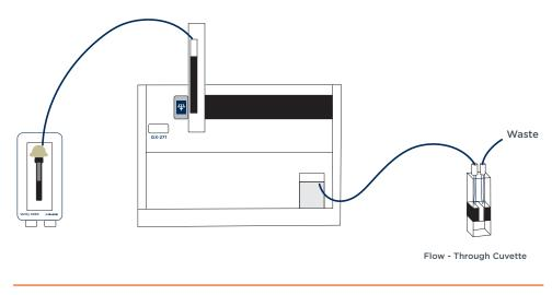
Figure 2 Transfer port configuration
