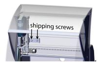
Shipping Screws (Front View of PIPETMAX\*)
