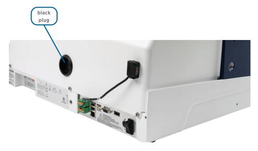
If your PIPETMAX does not have a rotating cover, it requires an external safety interlock. The external safety interlock was disconnected prior to running the alignment. Reconnect the BOTTOM terminal block connector to the input/output ports on the rear panel.
