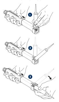
Take the following steps to ensure the DISTRITIP is correctly fitted:
