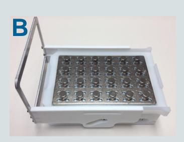
Custom magnetic bead separator used in the automated procedure. The handle of the device can be actuated by the liquid handler to move the magnets from the disengaged lower position (A) to the engaged upper position (B). When engaged, each magnet is in proximity to 4 wells of a 96 well plate.
